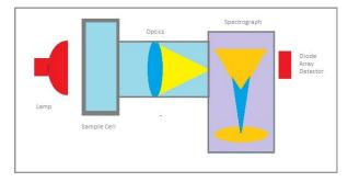
The light that passes through the sample is focused onto the entrance slit of the spectrograph which uses a stationary diffraction grating to separate the light into the frequency domain. The diffracted light is directed onto a silicon photodiode array detector where the intensity of the light is measured at each frequency. The intensity is related to the
